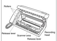
Follow steps 4 to 5 in Installing the ink film on p. 9, and close the operation panel.
